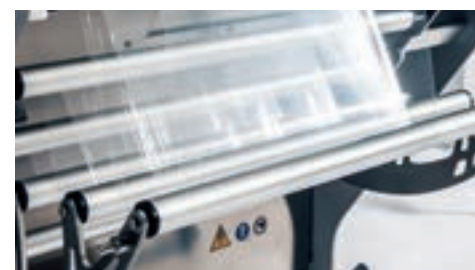
Optimised film unwinding and tensioning system
